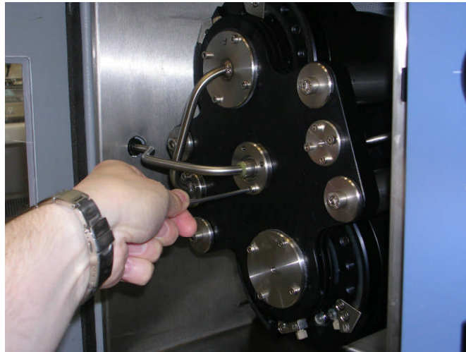
Figure 4 Detachment of Central Flying Lead Guide
